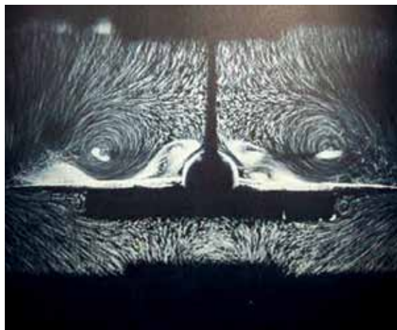
This photo of a model of the Concorde jet in a wind tunnel shows the vortices forming over the wings, as in the sketch by Leonardo (above right).
