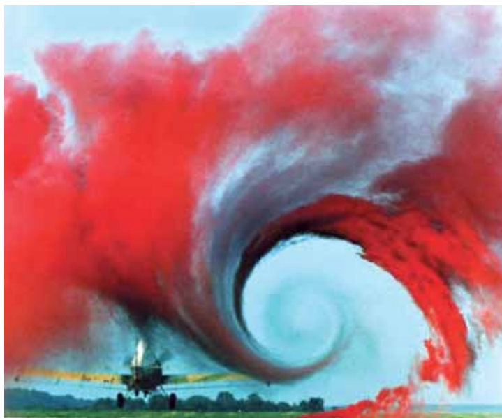
From a study of wake vortex formation at Wallops Island NASA Langley Research Center, 1990 (false color).
